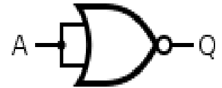
[NOT Gate by using NOR Gates only]
